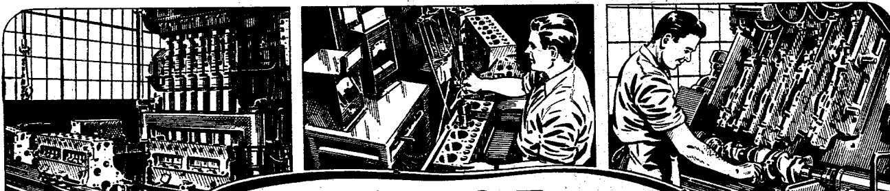
ABOVE — Superfinish honing of cylinder bores. Mirror-smooth finish assures long wear. CENTRE, ABOVE—Piston fitting is made accurate and easy when cylinder bores have successfully passed this "finish-and-bore test", using accurate electric indicator.
